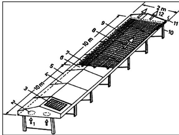
Figure 7.2 An illustration of solar tunnel drier (Kumar *et al.*, 2013).
