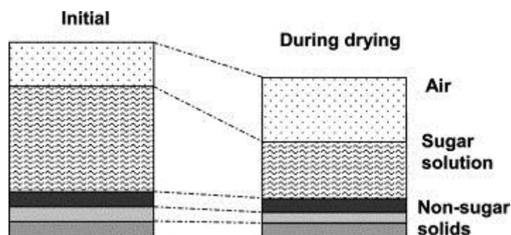
Figure 6.1 Different volumes in a porous medium with sugar molecules held in solution (May and Perre, 2002).
