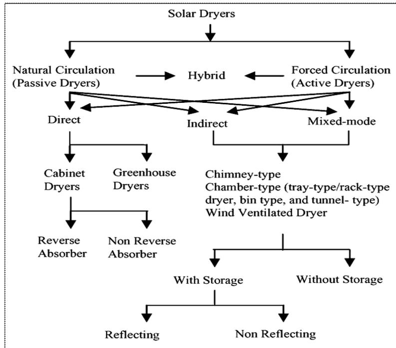
Figure 7.1 The classification of solar dryers (Fudholi *et al.*, 2010).
