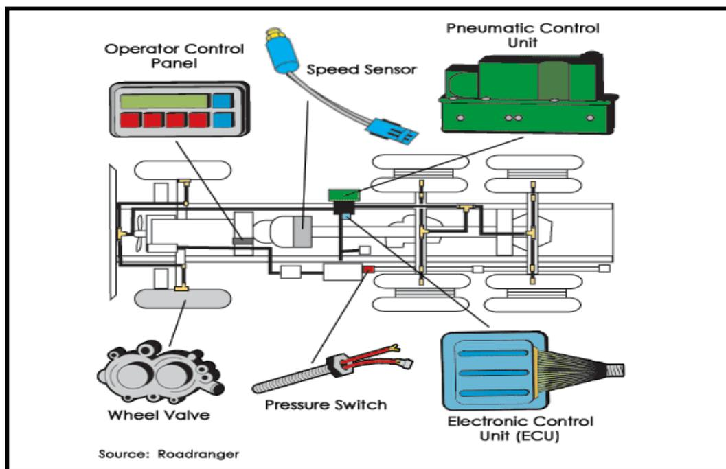
Figure 2. Components of a CTI system (Roadranger Vehicle Components, 2006).
