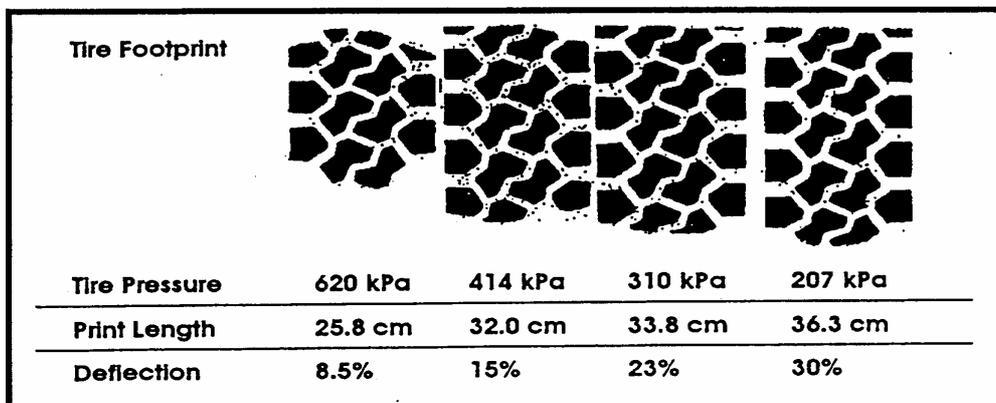
Figure 6. Tyre footprint and deflection with changes in tyre pressure (Bradley, 1996).
