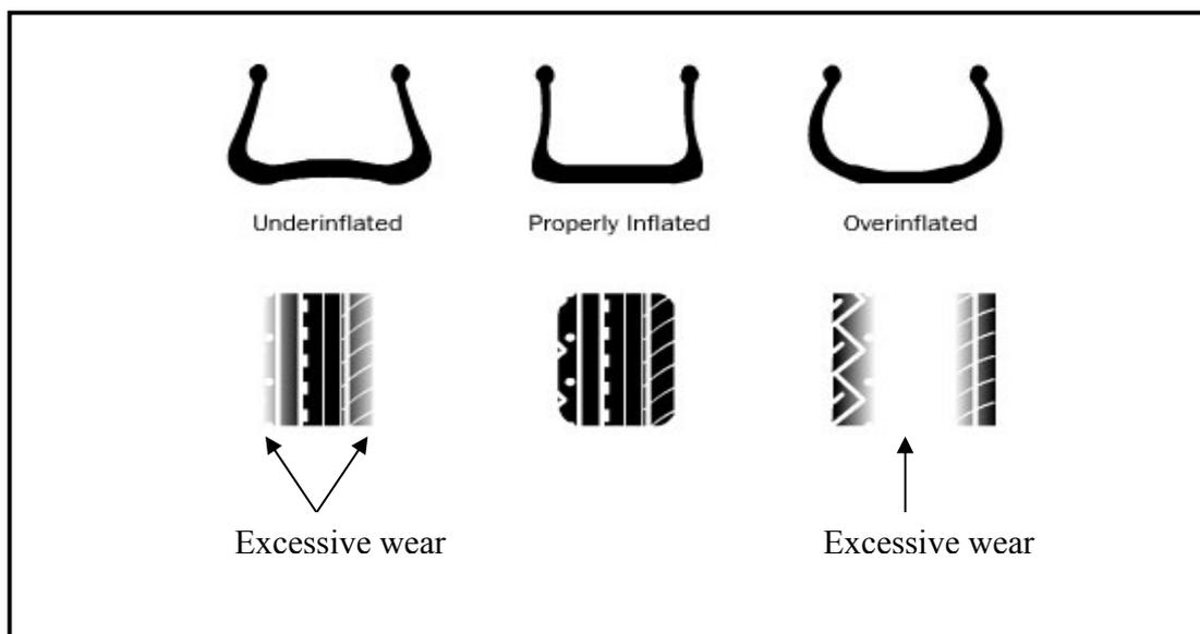
Figure 9. Illustration of excessive tyre wear when tyres are operated at incorrect pressures.
