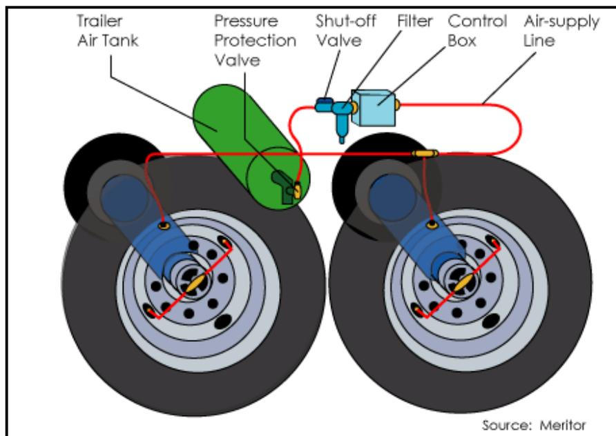
Figure 3. CTI air supply (Arvinmeritor Automotive Supplies, 2006).
