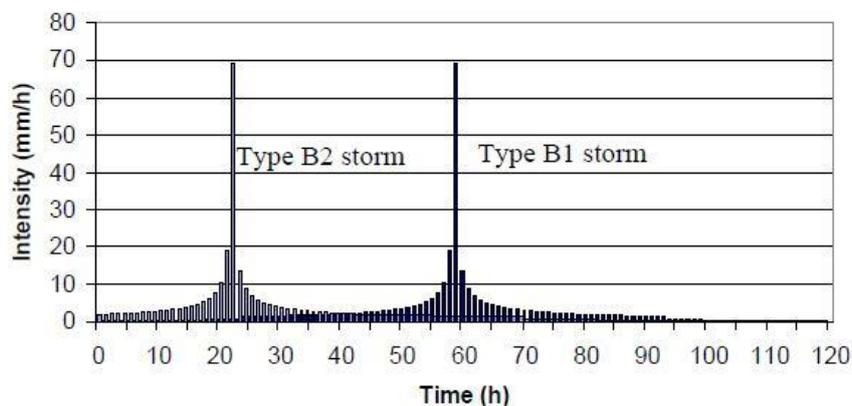
Figure 2.7 Example of design hyetographs derived from the ABM with a 1-hour timestep (Nguyen *et al.*, 2008)
