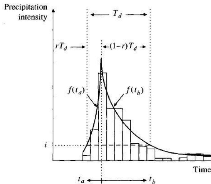
Figure 2.8 Fitting a curve to a hyetograph with the Instantaneous Intensity Method (Chow *et al.*, 1988)
