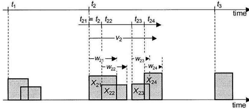
Figure 2.9 Schematic of the BLRP model process (Koutsoyiannis and Onof, 2001)
