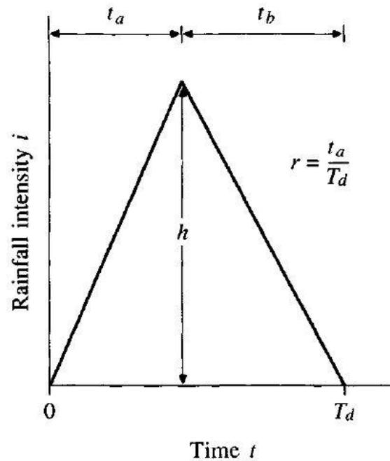
Figure 2.5 General model of the triangular distribution hyetograph (Chow *et al.*, 1988)
