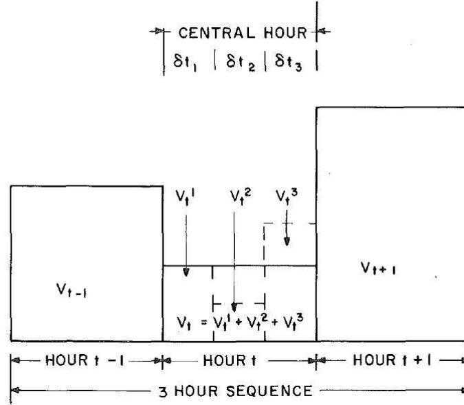
Figure 2.11 Discrete disaggregation model (Ormsbee, 1989)
