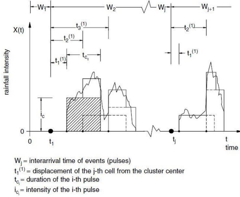
Figure 2.10 Schematic of the NSRP model process (Olsson and Burlando, 2002)
