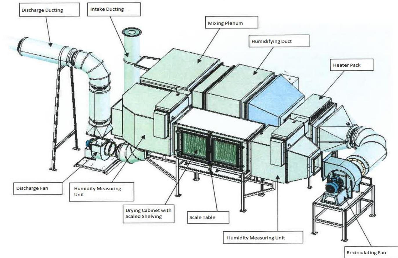
Figure 5.1 Layout of the laboratory drying unit
