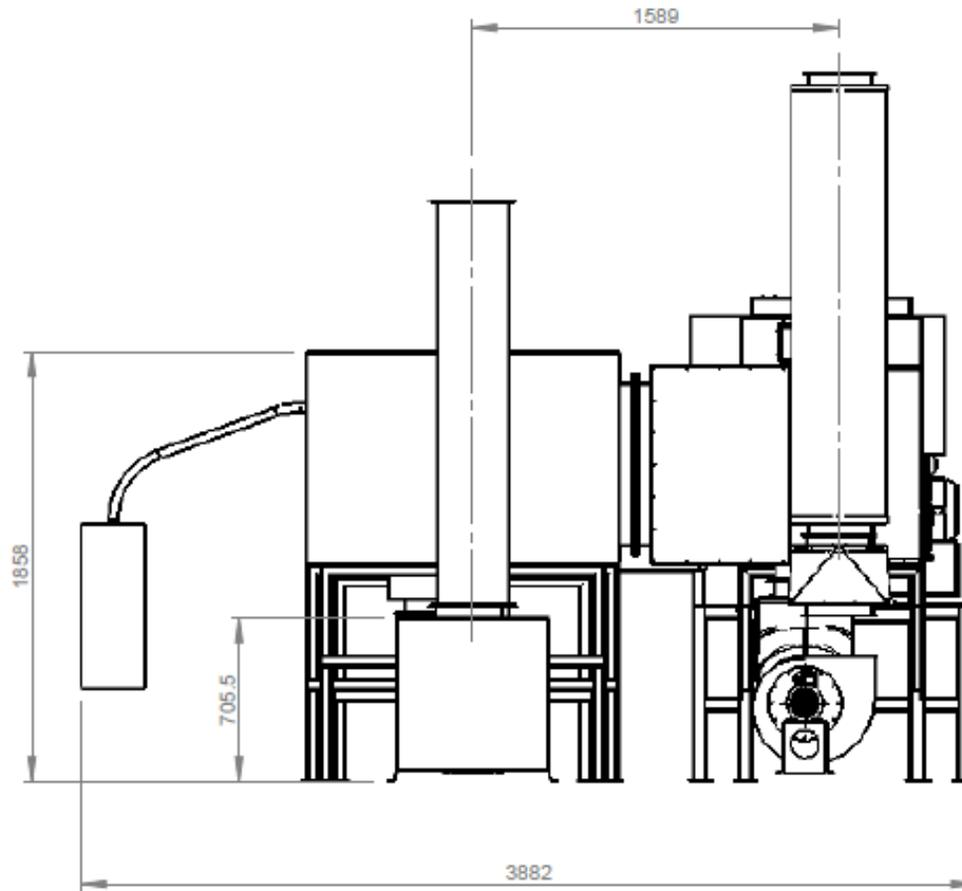
Figure 5.4 Left view of the laboratory drying unit
