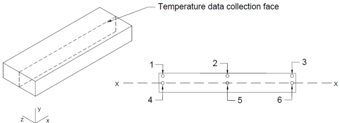
Figure 3.3 3D and 2D models of the meat sample showing the temperature data collection point; 1(20, 1), 2(75, 1), 3(130, 1), 4(20, 10), 5(75, 10), and 6(130, 10). X-X is the axis of symmetry.
