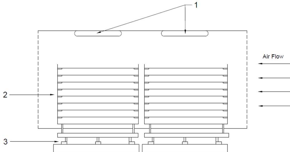
Figure 3.1 Schematic of the drying cabinet; 1 = IR halogen lamp heaters, 2 = Scaled shelving, 3 = Loads cells
