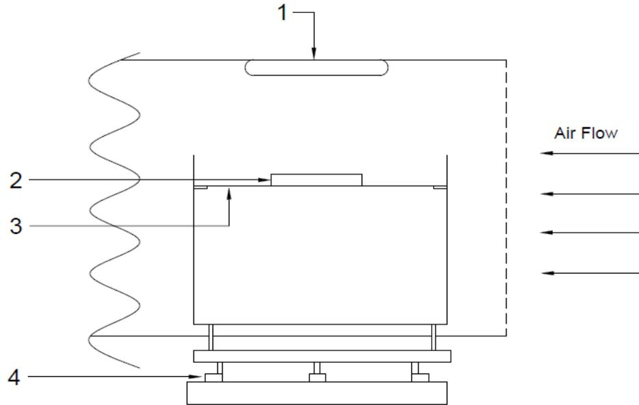
Figure 3.2 Set up of the drying experiment; 1 = IR halogen lamp heaters, 2 = Meat sample, 3 = Drying tray, 4 = Loads cells
