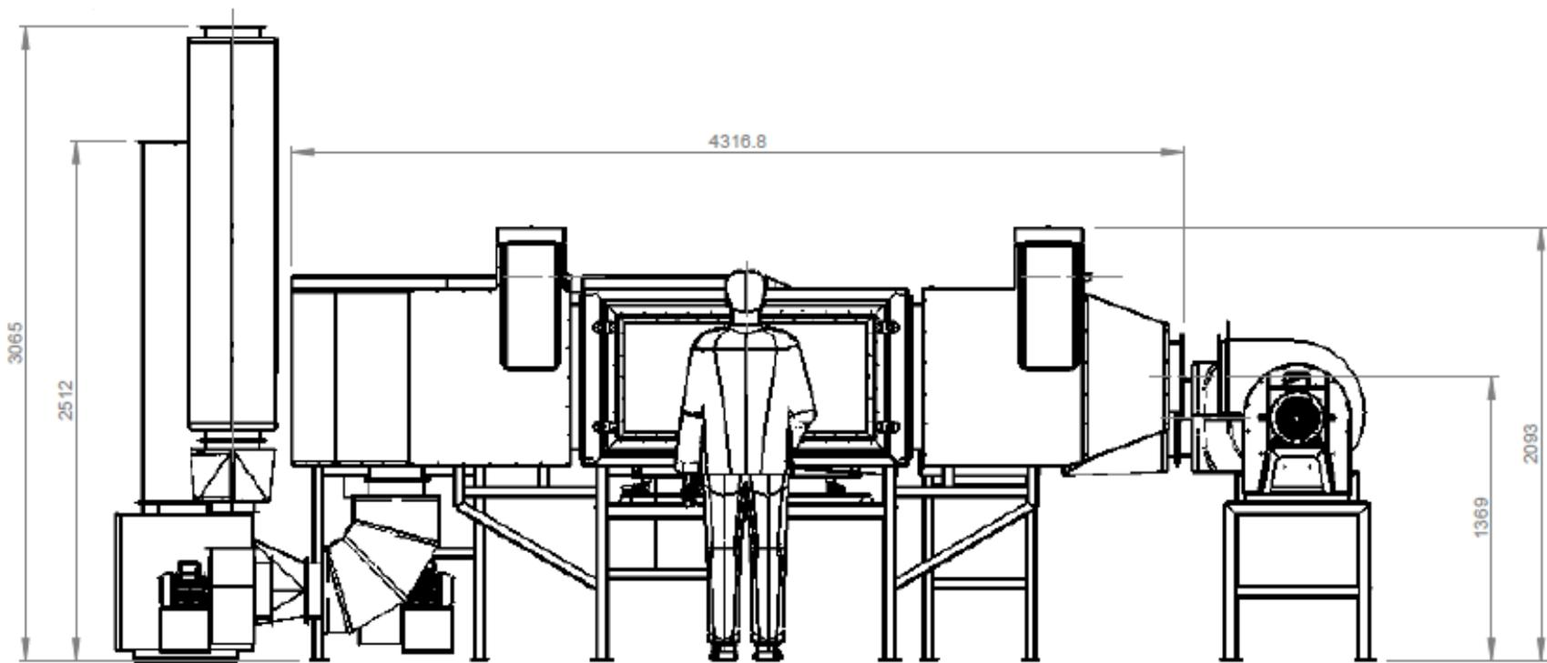
Figure 5.3 Front view of the laboratory drying unit
