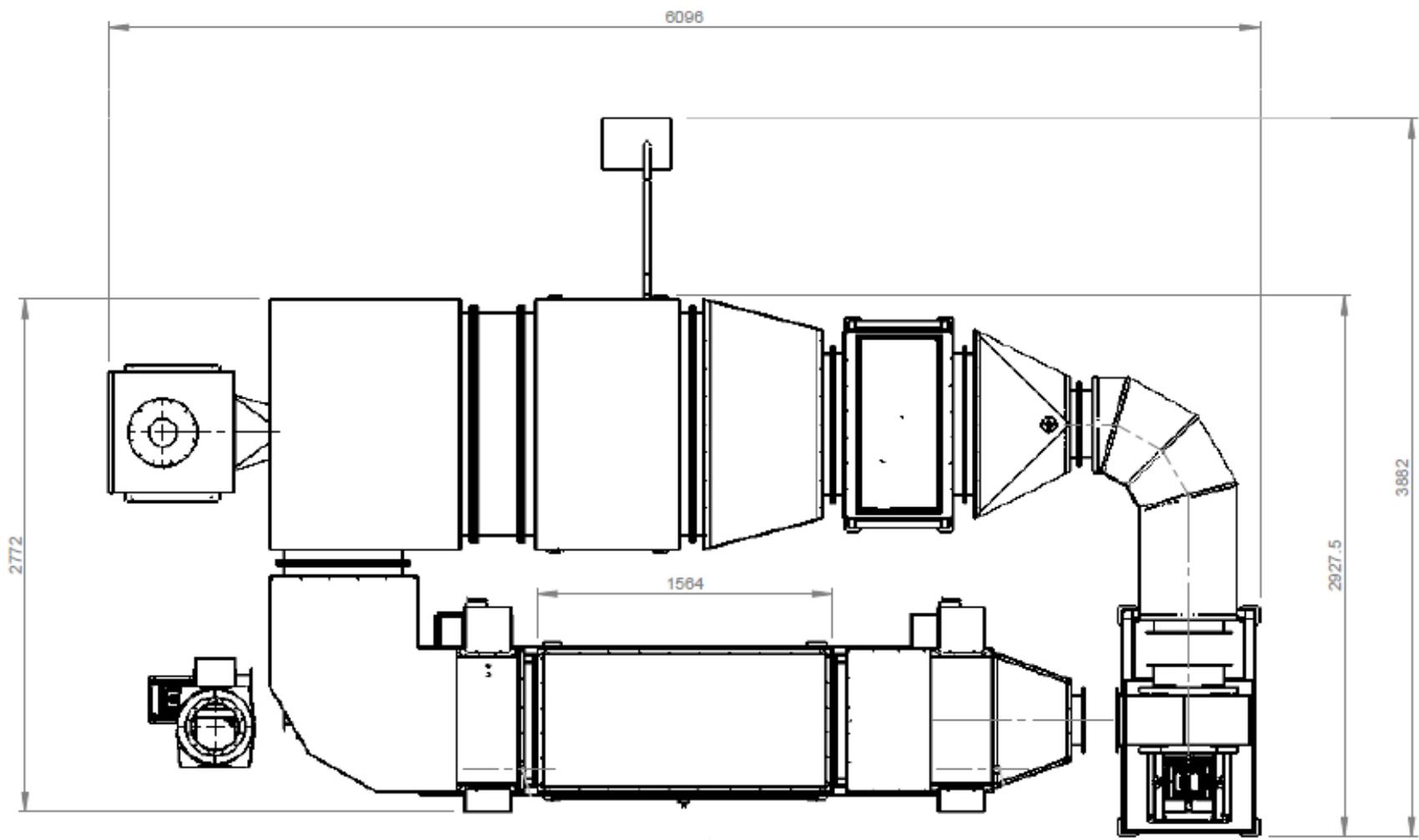
Figure 5.2 Top view of the laboratory drying unit
